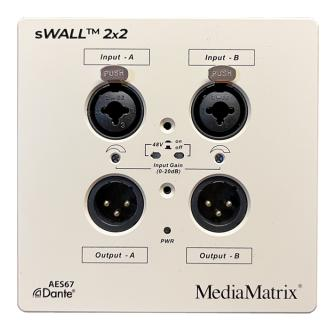
3.7 48v Phantom power micro switch LED is a self-locking button. When depressed status LED lights up indicating Phantom power is enabled.
