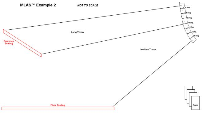
This line array could consist of a vertical coverage arrangement including a **Straight line** segment to cover the balcony, and a **Mild Angle** segment for the floor seating.
