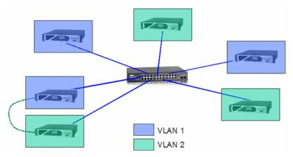
In this scenario, VLANs are configured using the port based VLAN capability of a managed switch.
