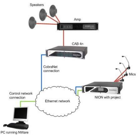
The control network and CobraNet network are both represented by a single *cloud*. You may choose to physically separate the wiring for the two networks, or logically separate the traffic using VLANs.
