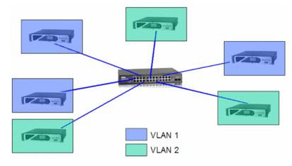
In this scenario, port based VLANs have been configured within a managed switch:
