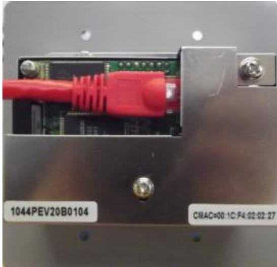
2. Carefully place the nWall into a 2-gang NEMA box.
