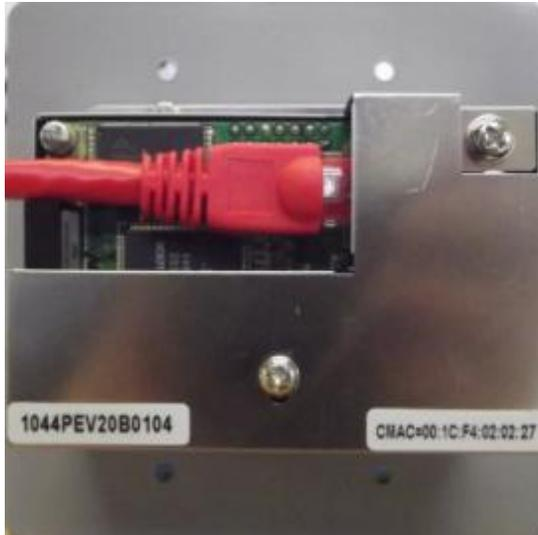
2. Carefully place the nWall into a 2-gang NEMA box.
