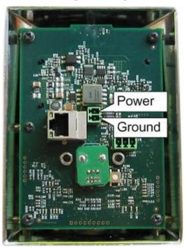
b) Insert the plug into the connector socket.
